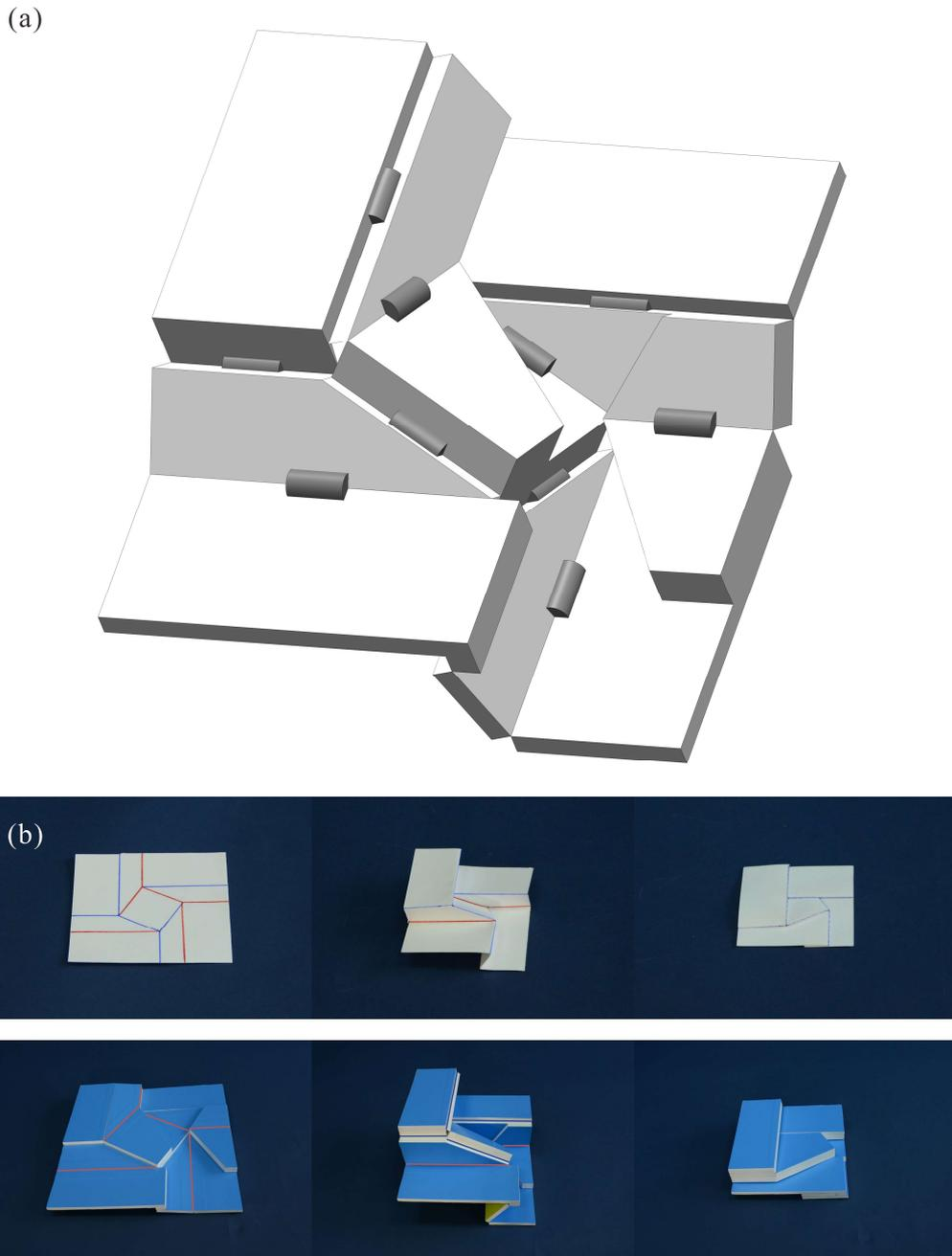
Figure 4-4 Thick panel models of square twist pattern, (a) Solidworks model for the square-twist pattern with thick panels, (b) zero-thickness model of square twist pattern and its corresponding thick panel model.
