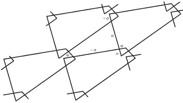
**Fig. 9** The schematic diagram of a grid-like assembly of equilateral Bennett linkages
