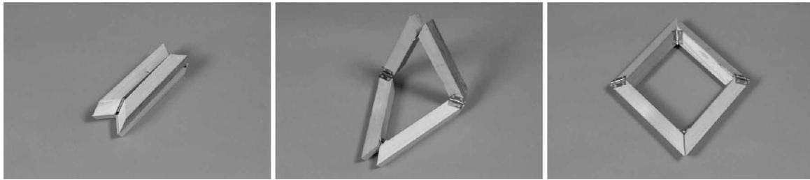
**Fig. 7** Expansion sequence of model 2 that opens up to a diamond shape
