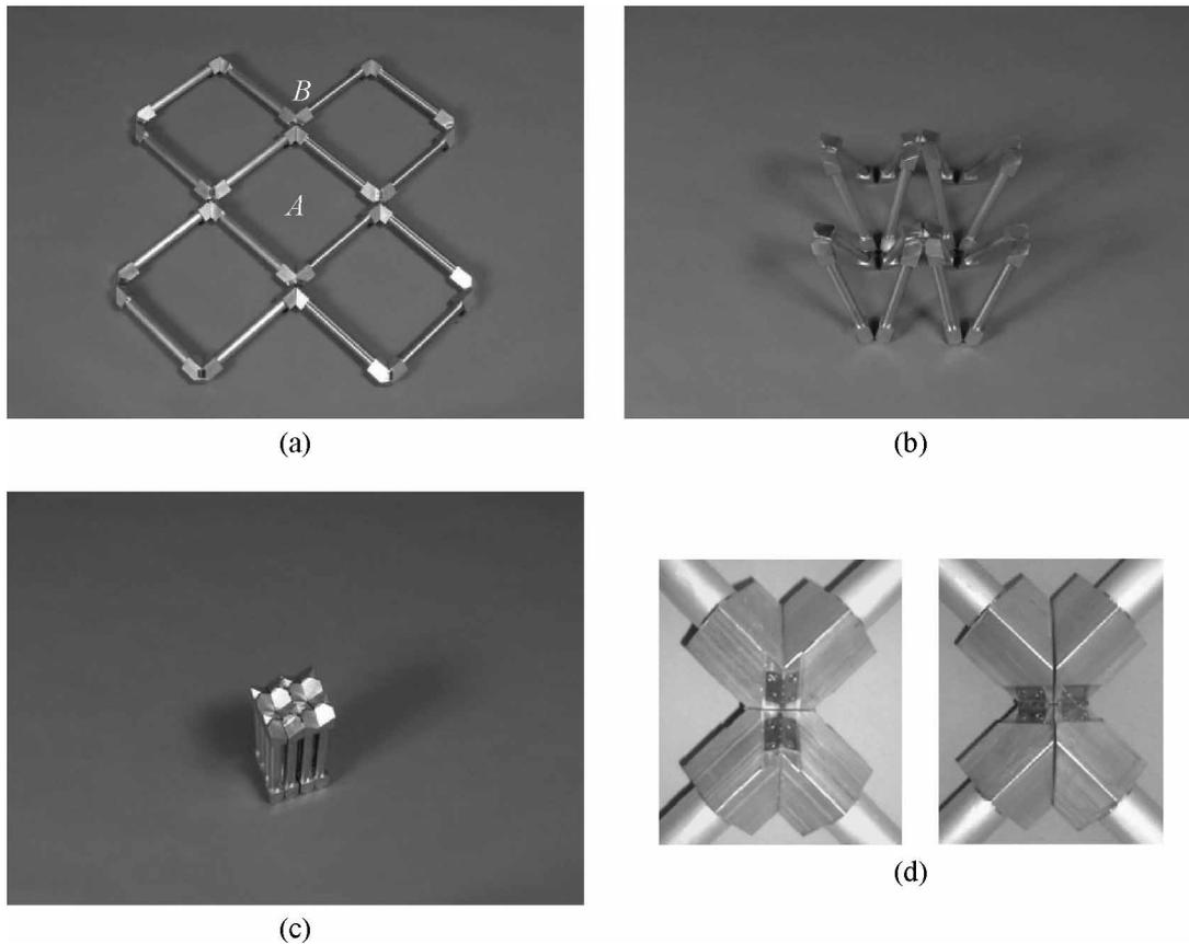
**Fig. 11** A model of assembly of the Bennett linkages in the alternative form. (a) to (c) Folding sequence of a model in the alternative form and (d) Front and rear views of the joints
