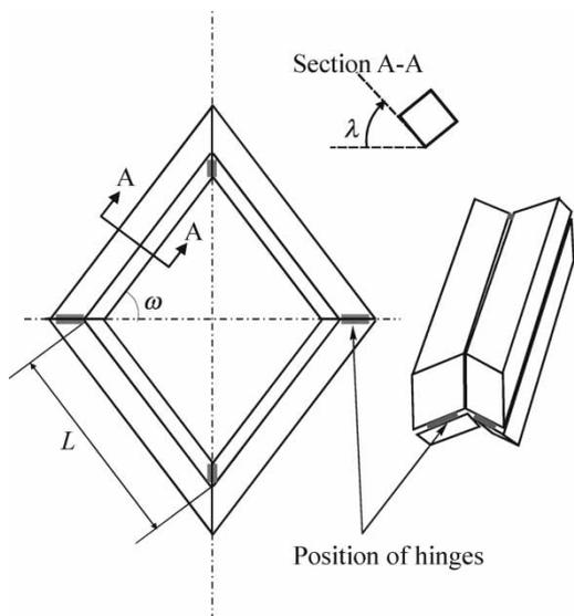
**Fig. 1** The alternative form of the Bennett linkage made from square cross-section bars in the deployed and folded configurations
