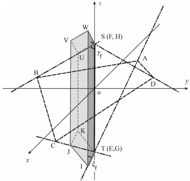
Fig. 5 The alternative form of the Bennett linkage with square cross-section bars in the folded configuration
