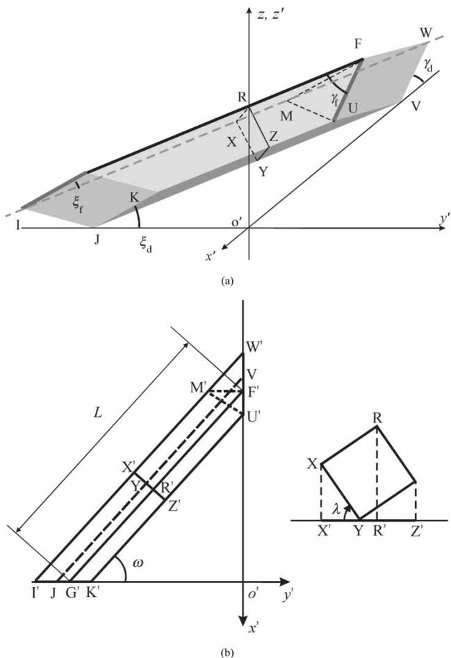
**Fig. 3** The geometry of the square cross-section bar: (a) in three-dimension and (b) projection on the plane  $x'o'y'$  and the enlarged cross-section  $RXYZ$
