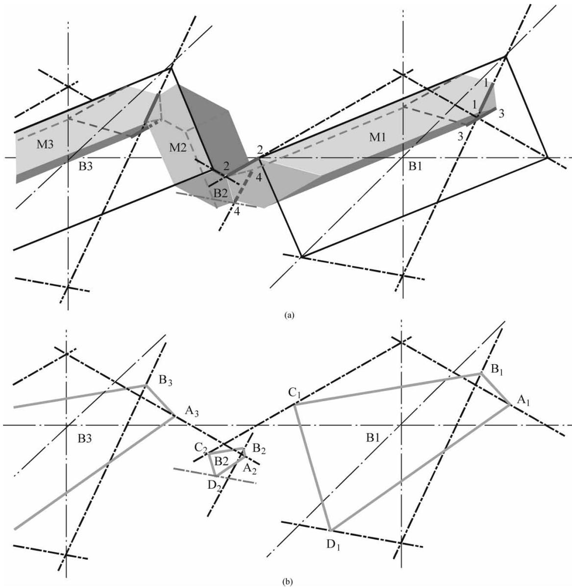
**Fig. 10** (a) The schematic diagram of a grid consisting of Bennett linkages in their alternative forms. Only one member is shown in each Bennett linkage. (b) The corresponding grid of original Bennett linkages
