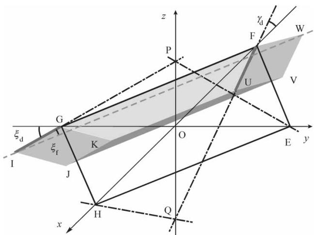
**Fig. 2** The alternative form of the Bennett linkage with square cross-section bars in the deployed configuration
