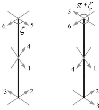
Fig. 6 The 6R linkages (a) for a given  $\alpha_{56}=\zeta$  and (b) when  $\alpha_{56}$  is increased to  $\pi+\zeta$
