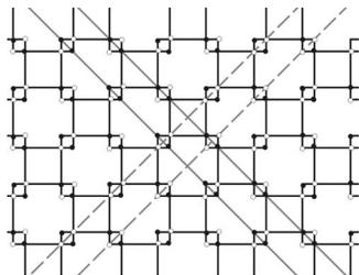
Fig. 9 A schematic diagram for an assembly of the new 6R linkages
