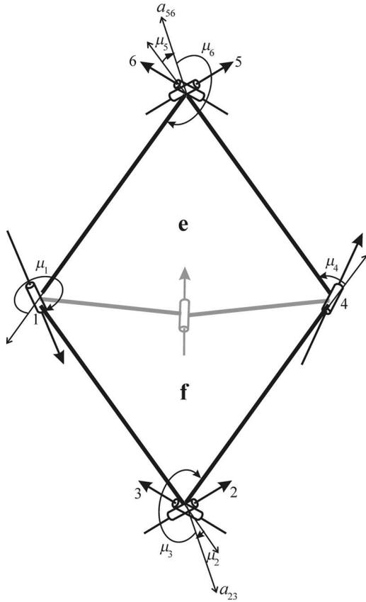
Fig. 4 A 6R linkage from two extended Myard linkages e and f
