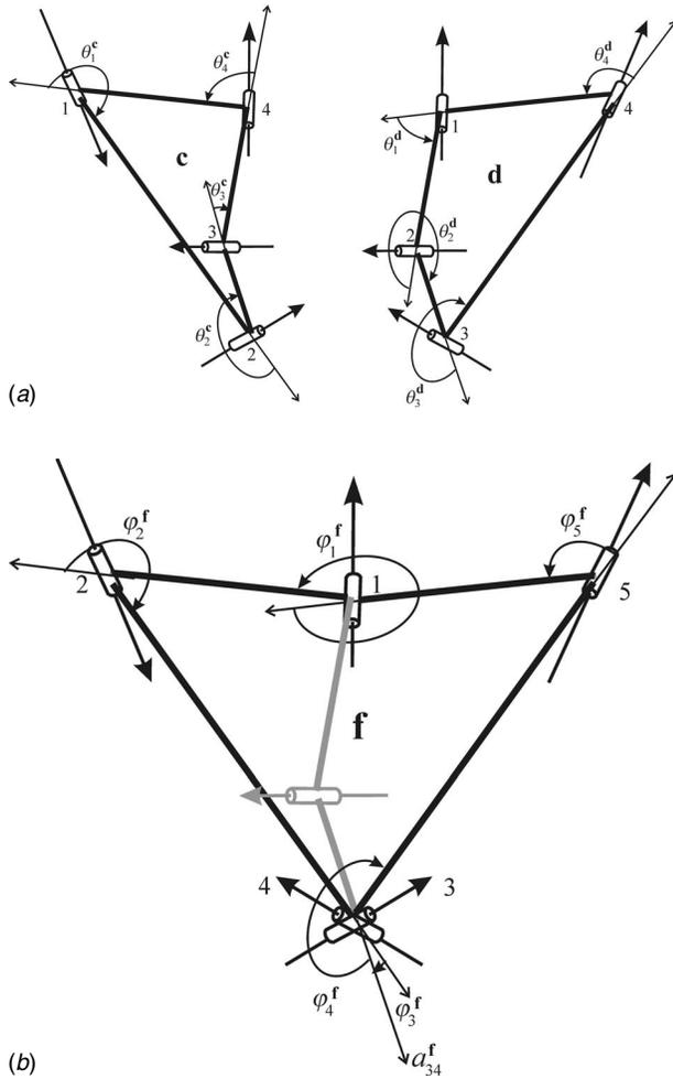
**Fig. 3** (a) Two Bennett linkages **c** and **d**. (b) They are combined to form an extended Myard linkage **f**.
