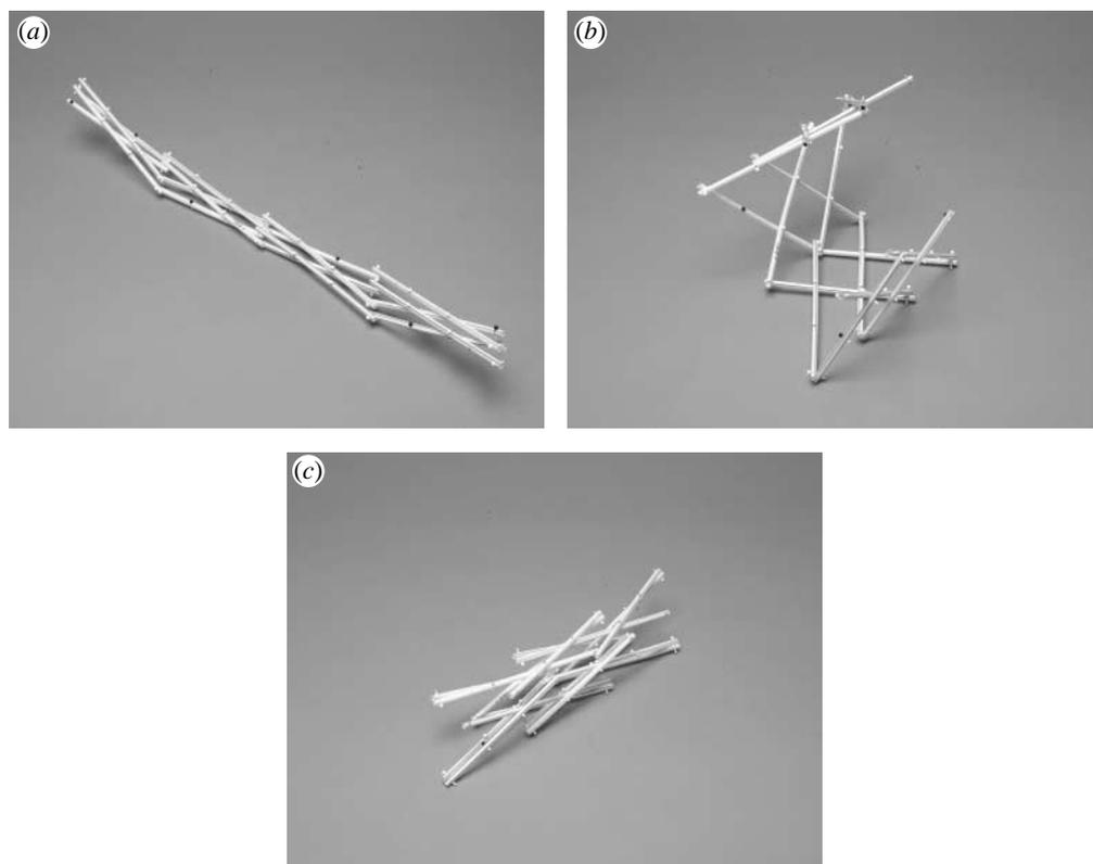
Figure 10. (a–c) Deployable sequence of a case 3 model.
