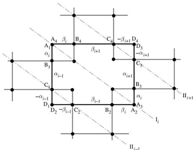
Figure 5. A typical Bennett linkage in a case 1 assembly.
