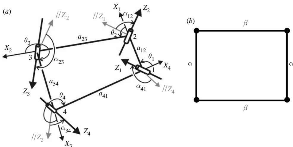
Figure 2. (a) A Bennett linkage and (b) its schematic.
