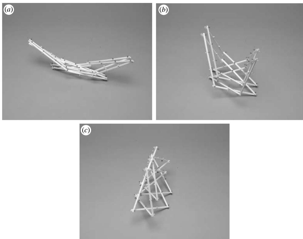
Figure 12. (a–c) Deployable sequence of a case 4 model.
