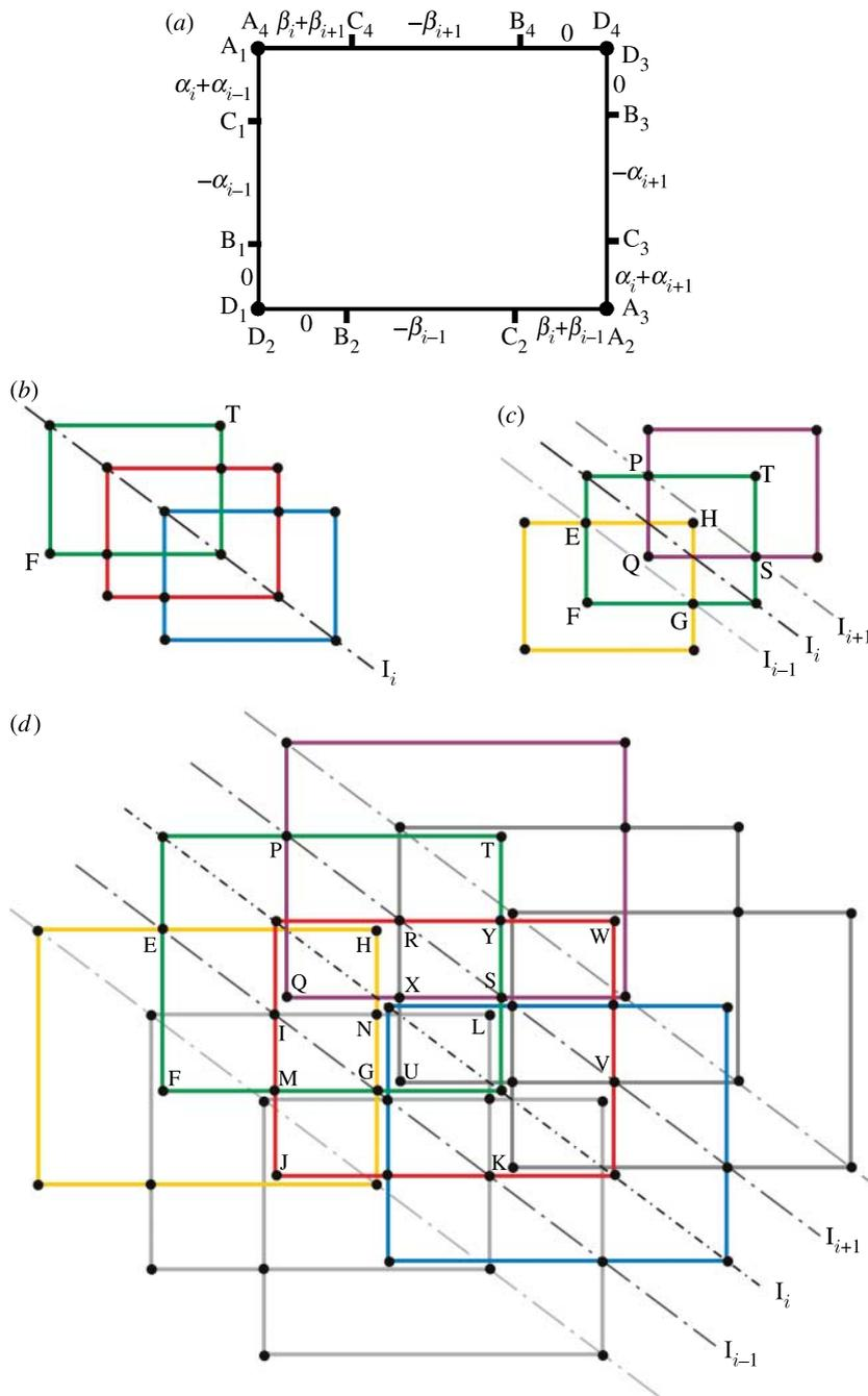
Figure 11. Construction of a case 4 assembly. (a) A basic unit. (b) Connection of linkages along the guideline and (c) in the other diagonal direction. (d) The whole assembly.
