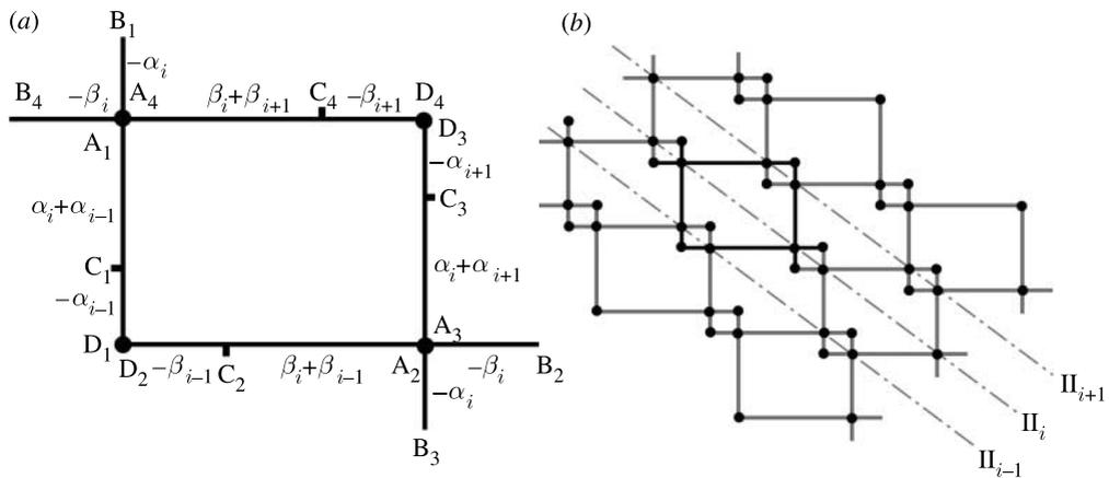
Figure 7. Construction of a case 2 assembly. (a) A typical linkage and (b) its assembly.
