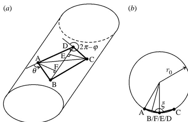
Figure 18. The geometry of a single Bennett linkage. (a) On the surface of a cylinder and (b) the cross-section view.
