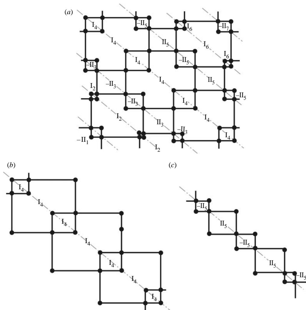
Figure 3. Schematic of assembly of similar Bennett linkages and its guidelines. (a) Whole assembly, (b) linkages on type I guideline and (c) linkages on type II guideline.
