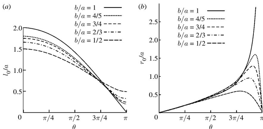
Figure 19. The geometrical parameters of a Bennett linkage when  $\alpha = \pi/3$ . (a)  $l_0/a$  versus  $\theta$  and (b)  $r_0/a$  versus  $\theta$  for various  $b/a$ .
