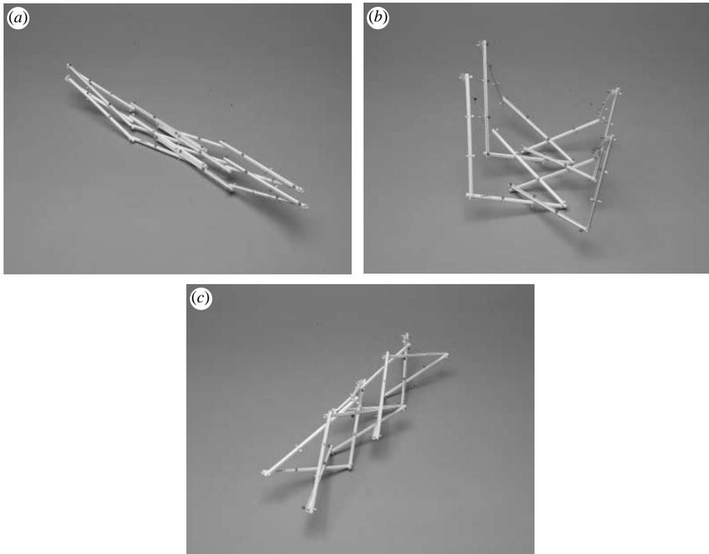
Figure 6. (a–c) Deployment sequence of a case 1 model.
