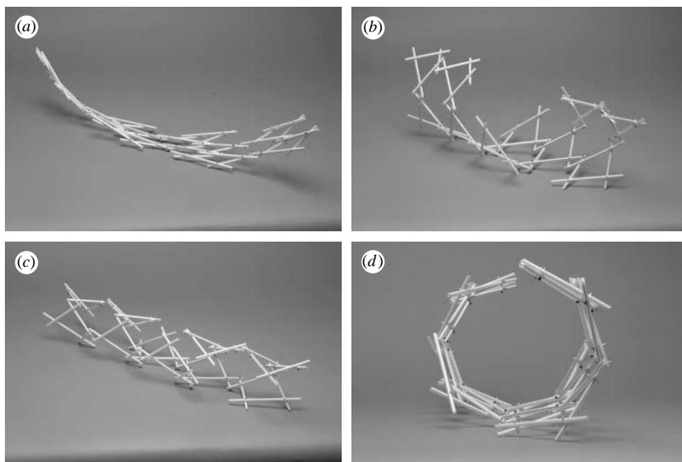
Figure 1. (a–c) Expansion sequence of an assembly based on the Bennett linkage and (d) the sectional view of the assembly.
