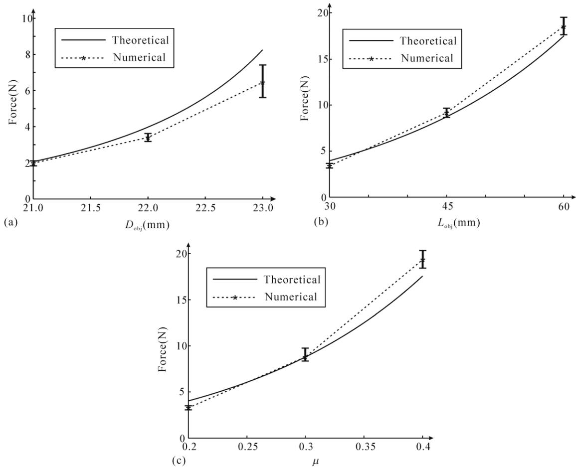
**Fig. 11** Effects of the properties of the object: (a) object diameter; (b) object length; (c) friction coefficient
