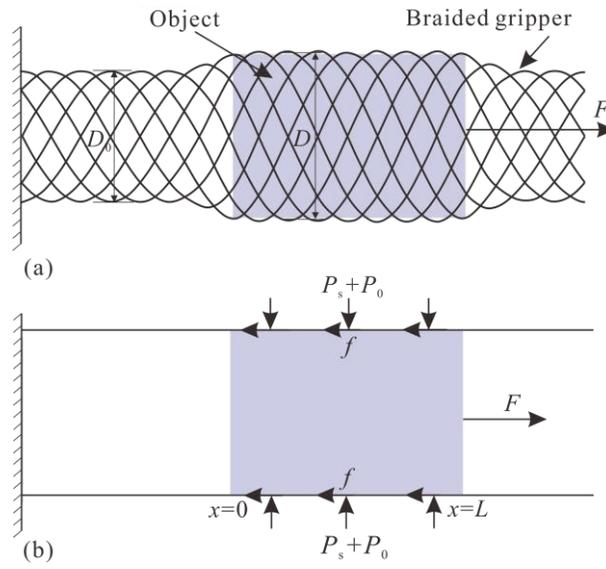
**Fig. 5** (a) Schematic and (b) force diagram of the gripper's grasping.
