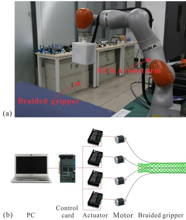
**Fig. 7** (a) The braided gripper mounted on a KUKA robot arm; (b) Actuation system.
