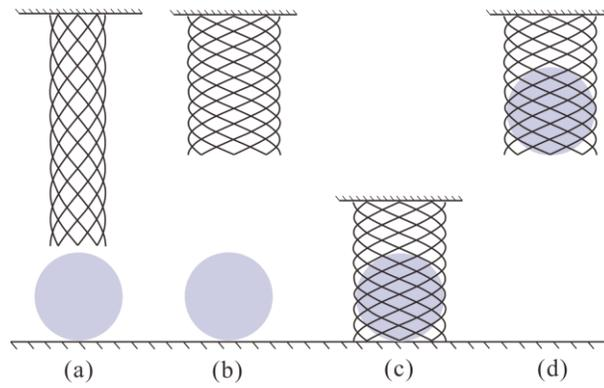
**Fig. 2** Grasping procedure of the braided gripper: (a) the normal state; (b) deployment of the gripper; (c) containing the object; (d) lifting the object
