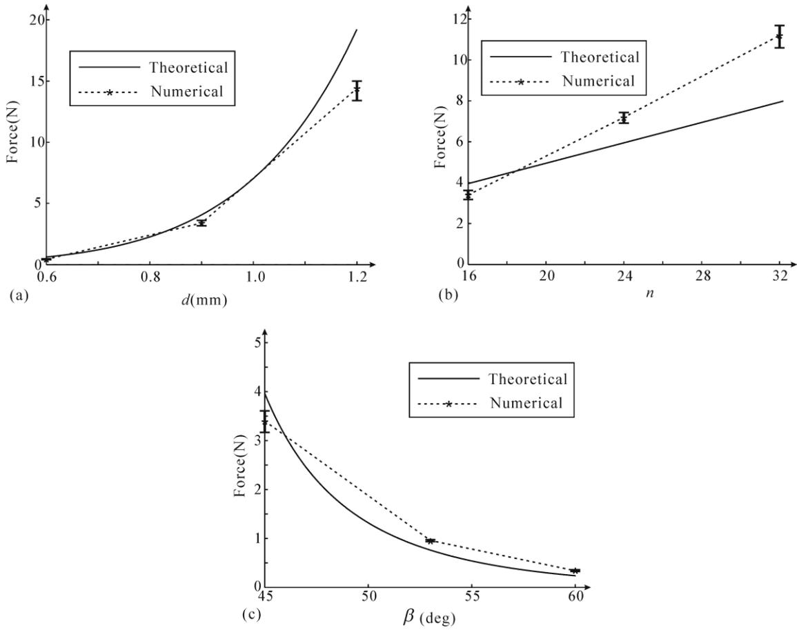
**Fig. 10** Effects of the properties of the gripper: (a) fiber diameter; (b) fiber number; (c) braiding angle
