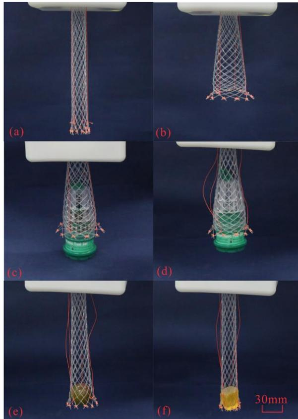
**Fig. 12** The braided gripper (a) in the normal state; (b) in the deployed state; (c) contains the object; (d) lifts the object; (e) grasps the grape; (f) grasps the jelly.
