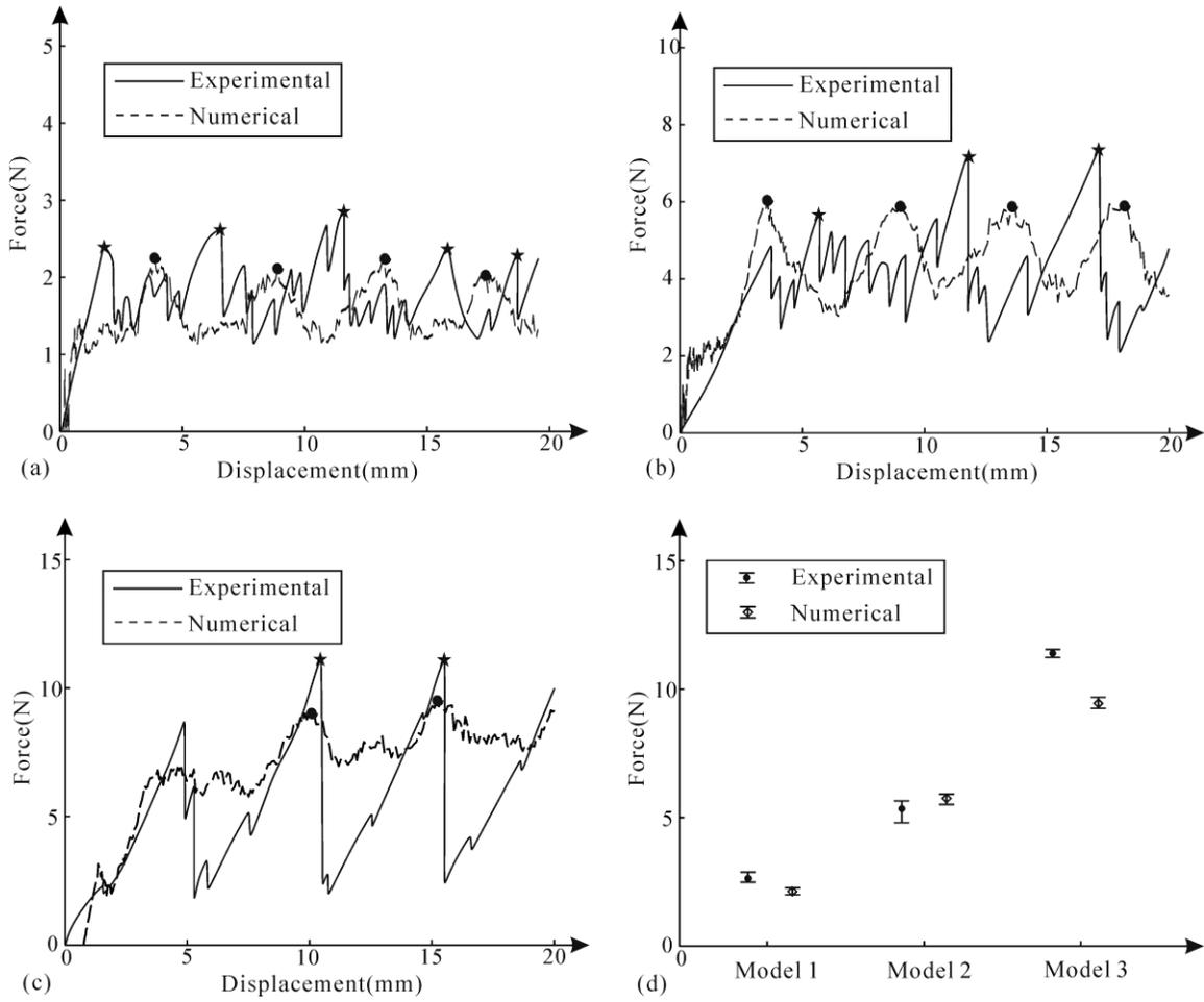
**Fig. 9** Experimental and numerical displacement versus force curves of the gripper grasping objects with (a)  $D_{obj}=19.8\text{mm}$ ,  $L_{obj}=20\text{mm}$ , (b)  $D_{obj}=21.8\text{mm}$ ,  $L_{obj}=20\text{mm}$ , and (c)  $D_{obj}=21.8\text{mm}$ ,  $L_{obj}=30\text{mm}$ , and (d) their error bars representing extrema
