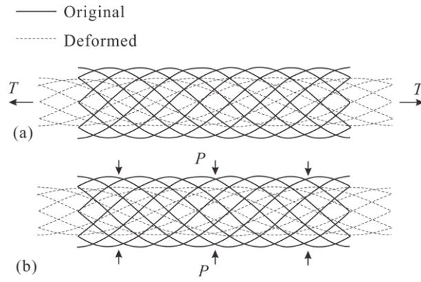
**Fig. 4** Elongation of a braided gripper at (a) tension force and (b) radial pressure.
