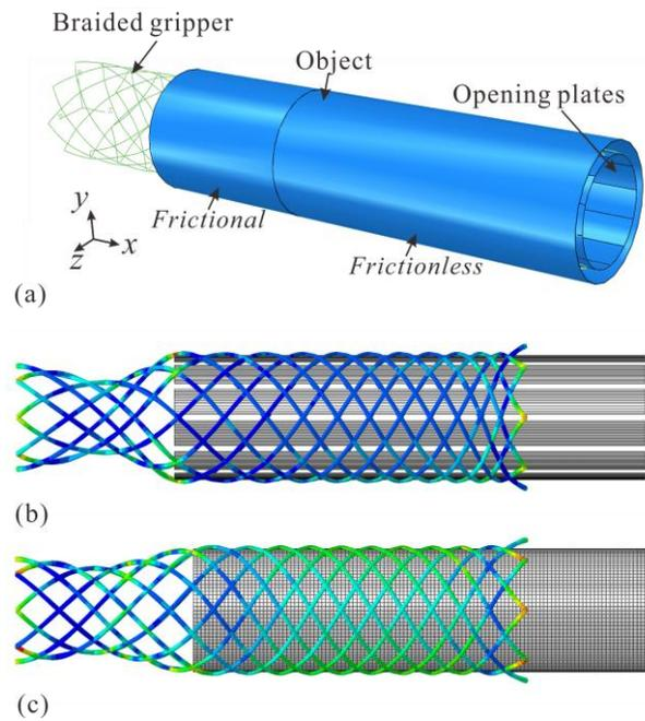
**Fig. 8** Finite element model: (a) Assembly of the model; (b) Deploying of the gripper with opening plates; (c) Moving the object in longitudinal direction.
