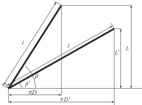
**Fig. 3** Spreading of a helical fiber in plane.
