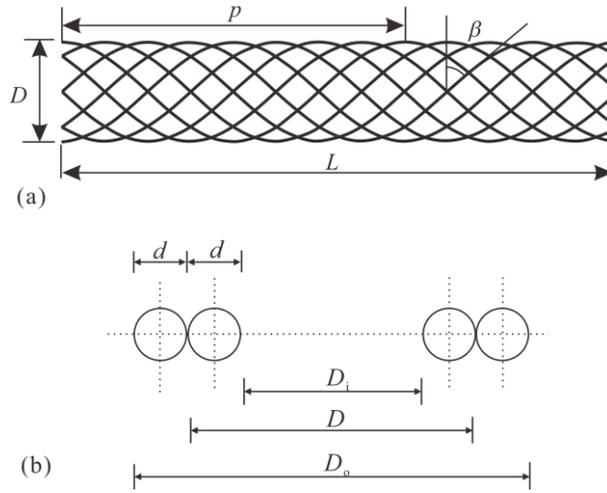
**Fig. 1** Geometry of the braided gripper.
